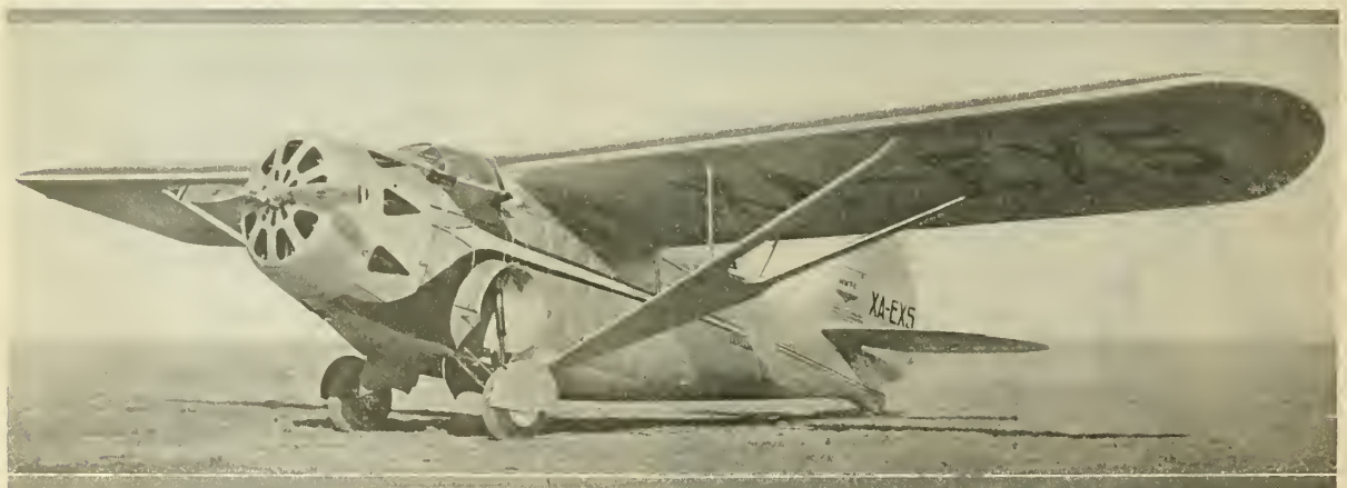
P. & W. Wasp-powered MWT-1 designed by Dr. Michael Watter and built in Mexico for long-range flight
